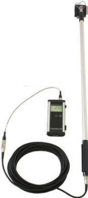
The SWT 316 is a measuring probe that is specially designed to measure surface temperature of rotating cylinders in a paper machine. This manual is also valid for SWT 315 (earlier model).
