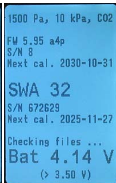
The same start-up information is displayed, with the addition of information about the external sensor, in this case an SWA 32.
