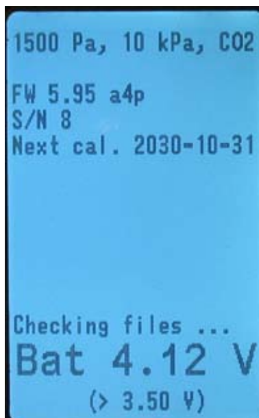
Two built-in pressure sensors and one built-in CO 2 sensor.
